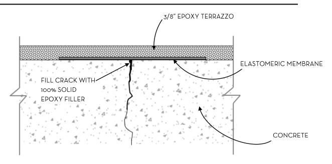
Concrete Crack Detail (Exceeding 1/16" in width)
