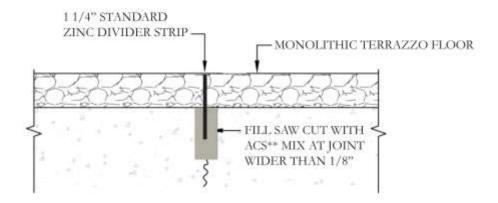
\*Care should be taken by concrete contractor to provide a straight joint, placed in coordination with design teams consideration of final grid pattern. Square edges encouraged, tooled edges discouraged.
