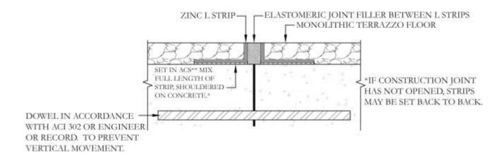
\*Care should be taken by concrete contractor to provide a straight joint, placed in coordination with design teams consideration of final grid pattern. Square edges encouraged, tooled edges discouraged.
