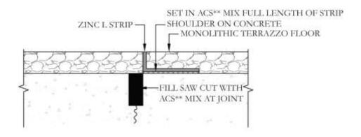
\*Care should be taken by concrete contractor to provide a straight joint, placed in coordination with design teams consideration of final grid pattern. Square edges encouraged, tooled edges discouraged.
