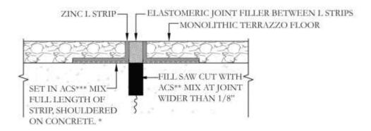
\*Care should be taken by concrete contractor to provide a straight joint, placed in coordination with design teams consideration of final grid pattern. Square edges encouraged, tooled edges discouraged.
